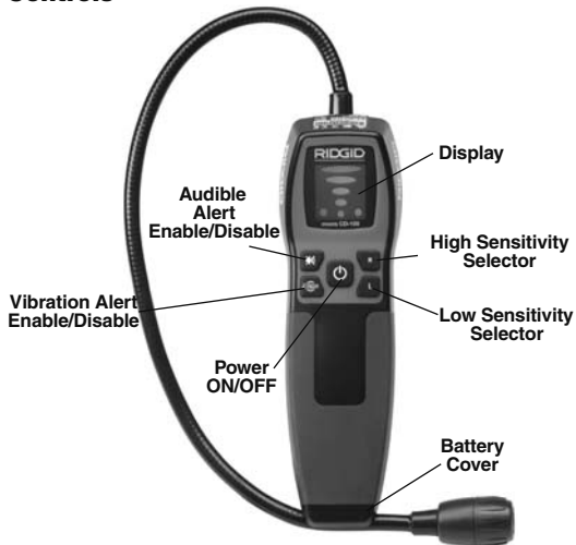
Figure 2 – micro CD-100 Parts
