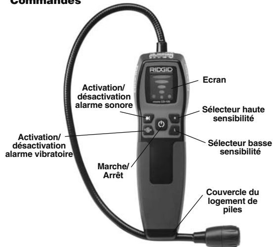
Figure 2 – Composants du micro CD-100
